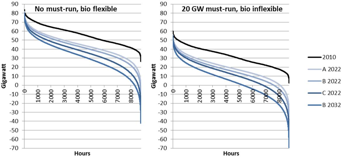
Figure 3: Residual load in NEP scenarios (reference load, means)
